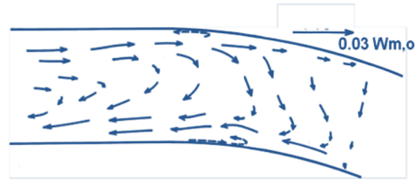
Figure 7. Steady streaming in horizontal plane ( D=300, Rc=10 ).
